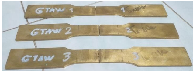
Figure 6. Tensile Test Results of Gas Tungsten Arc Welding Specimens
