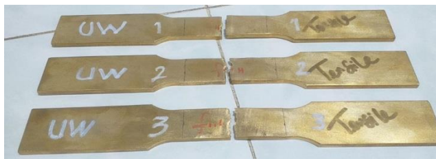
Figure 7. Tensile Test Results of Underwater Welding Specimens
